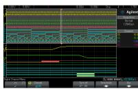
Signal details are lost with short record length and low sample rate.
